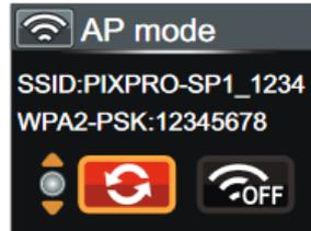
3. Open the WiFi settings on the Android tablet and connect to this WiFi network (PIXPRO-SP1\_1234 in this example)
